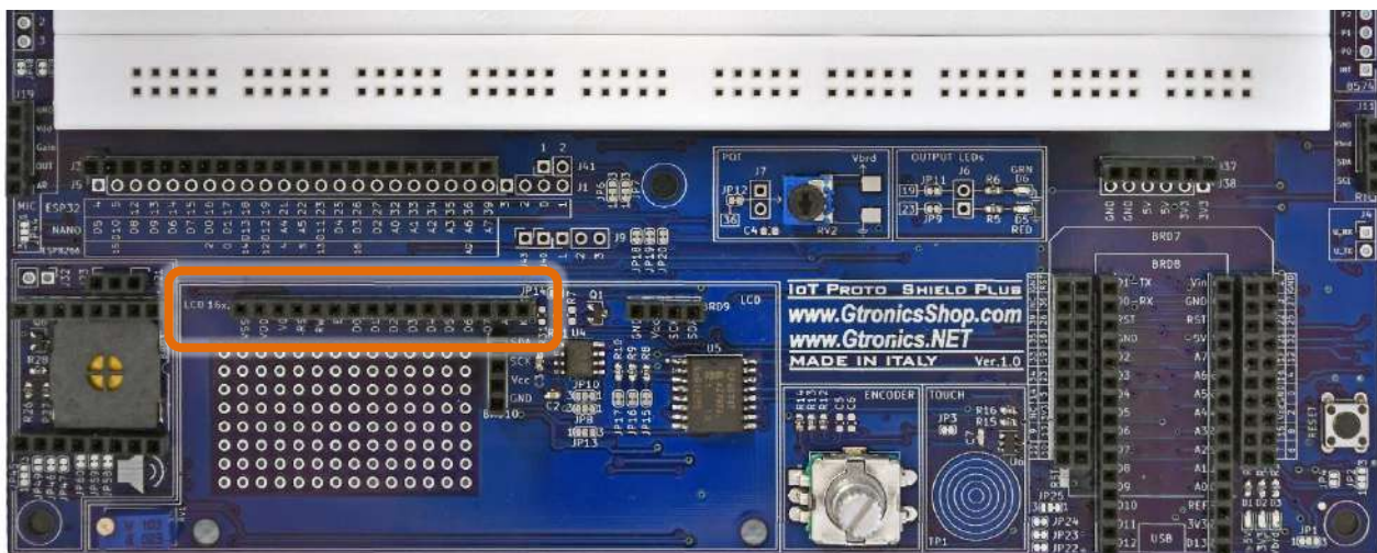
Figure 34 – Header LCD 16x2 della IOT PROTO SHIELD PLUS
