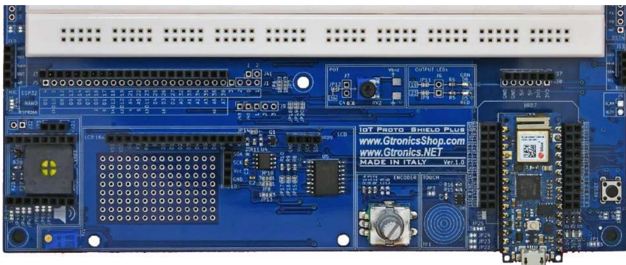
Figure 10 – An ARDUINO NANO (NANO33 IoT) plugged into the IoT PROTO SHIELD PLUS
