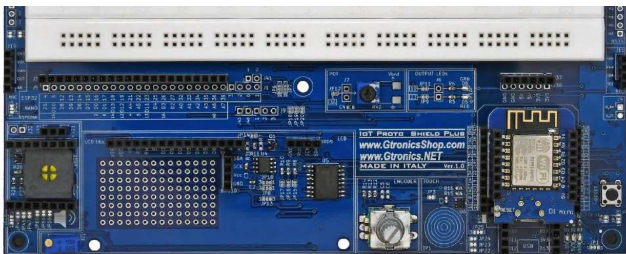
Figure 14 – The ESP8266 D1 mini plugged into the IoT PROTO SHIELD PLUS
