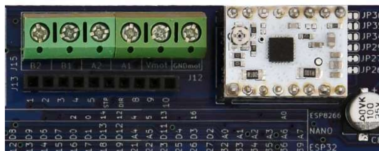
Figure 96 – A DRV8834 module plugged into BRD2 socket
