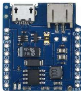
Figure 111 – Typical battery shield of widespread use
