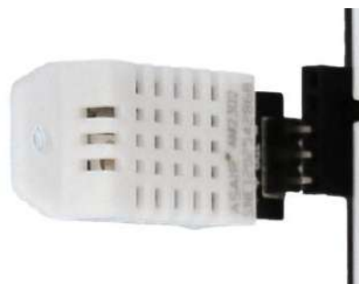
Figure 48 – A DHT22 module plugged into J31 of the IoT PROTO SHIELD PLUS
