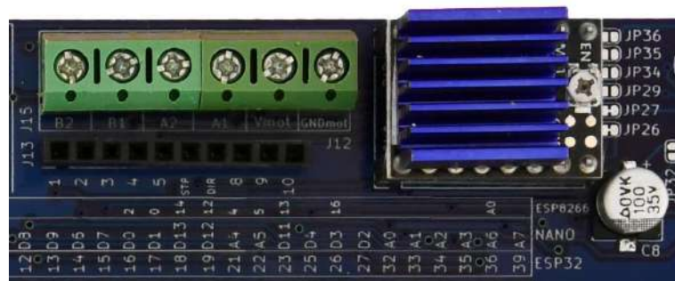
Figure 94 – A TMC2xxx module plugged into BRD2 socket
