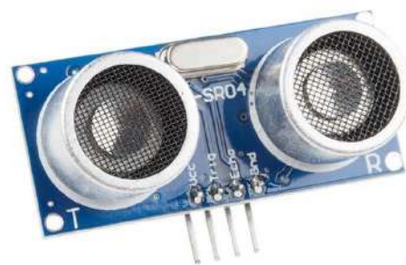
Figure 81 – HC-SR04 module of widespread use
