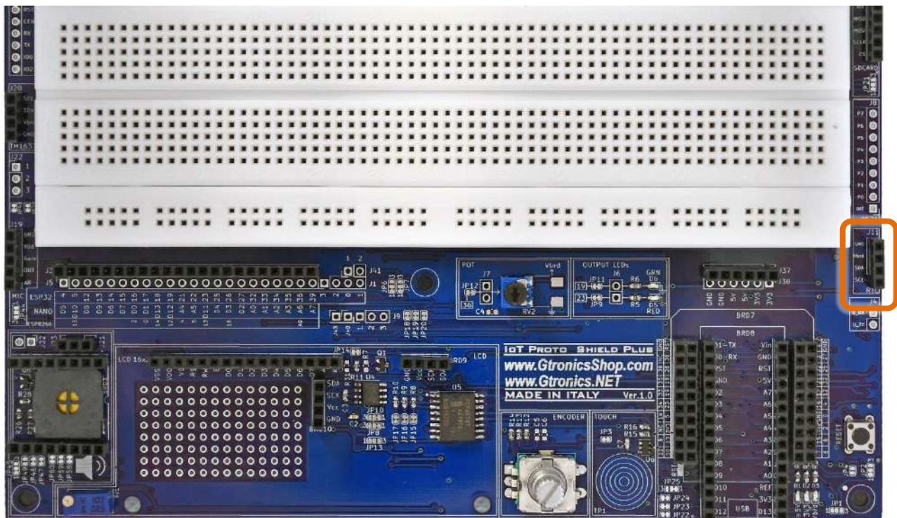
Figure 52 – J11 RTC header of the IOT PROTO SHIELD PLUS
