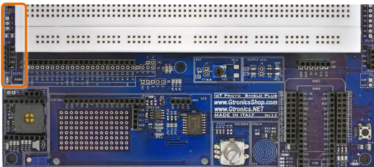
Figure 72 – MIC section of the IOT PROTO SHIELD PLUS
