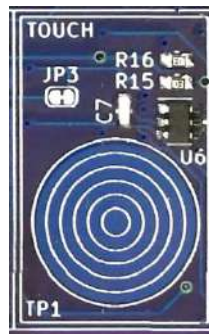
Figure 24 – TOUCH section of the IoT PROTO SHIELD PLUS
