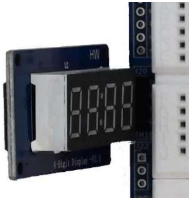
Figure 40 – An TM1637 digital display module plugged into J20 header of the IOT PROTO SHIELD PLUS
