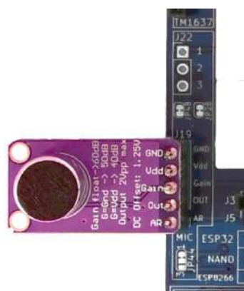
Figure 74 – A MAX9814 microphone plugged into J19
