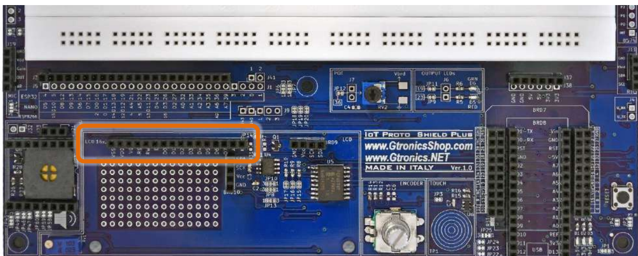
Figure 34 – LCD 16x2 header of the IOT PROTO SHIELD PLUS
