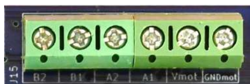
Figure 89 – J15 screw connector of the IoT PROTO SHIELD PLUS
