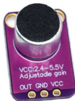
Figure 75 – A MAX4466 microphone module of widespread use
