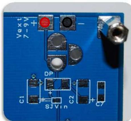
Fig. 31 – External power pads on the bottom of the board
