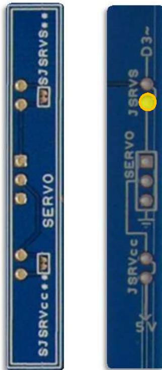
Fig. 28 – SERVO bottom and top board view
