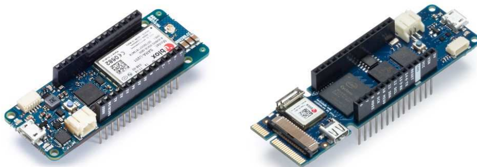
Figure 7 – Arduino MKR GSM 1400 and MKR Vidor 4000, both with stackable headers
